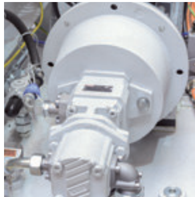
Frequency controlled hydraulic pump
