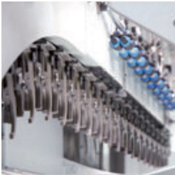
Tool magazine basic module with extension module in HSK-A63 version
