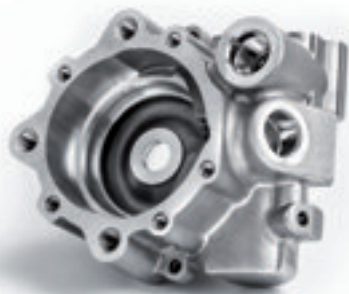
Servo pump housing 2-spindle solution with 4 parts clamping Machining in one clamping Machining time less than 82 s per workpiece
