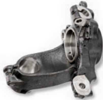
Cast iron knuckle (Front axle) Machining with 3 or 4 spindles in one clamping Machining time on the 3-spindle solution: 97 s per part Right and left workpieces are produced in the same machine
