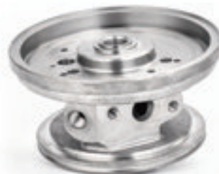
Bearing housing 2-spindle solution with a 4 part clamping fixture Machining of OP 20 after the turning process Part time less than 90 s possible
